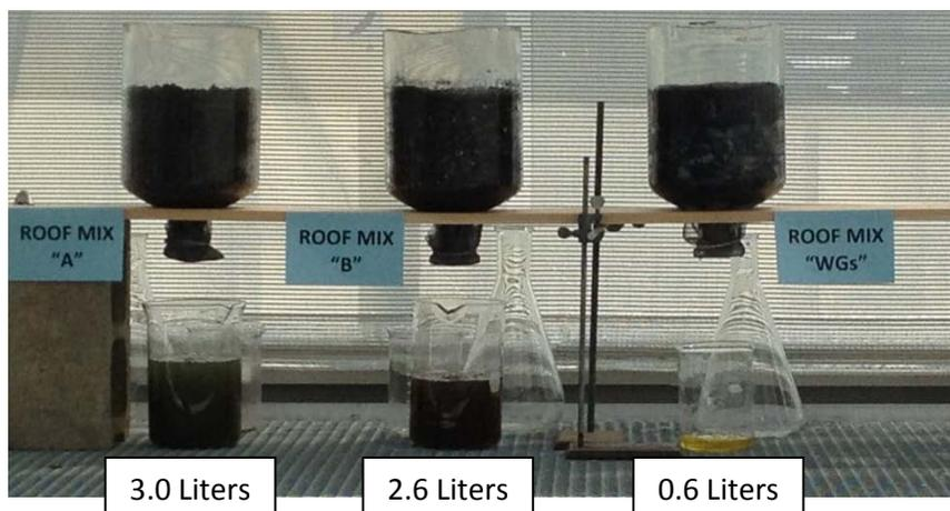
Figure 2. Comparison of two green roof materials planted the same day with plugs, conventional Norlite roof mix left, and Water Grip Brownies right box (October 2012).
